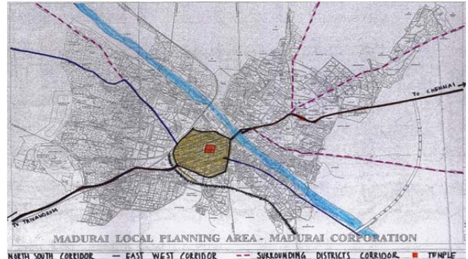
Fig. 3: Transport Corridors of the Madurai LPA region
